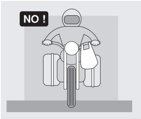
Absolutely do not hang bulky, voluminous, heavy and/or dangerous objects on the handlebar, the mudguards and the forks, as the vehicle could react more slowly in turns and its manoeuvrability could be unavoidably impaired. Do not place too bulky bags on the vehicle sides and do not hang the crash helmet from the apposite string, as they could hit people or obstacles, thus causing the loss of control of the vehicle.
